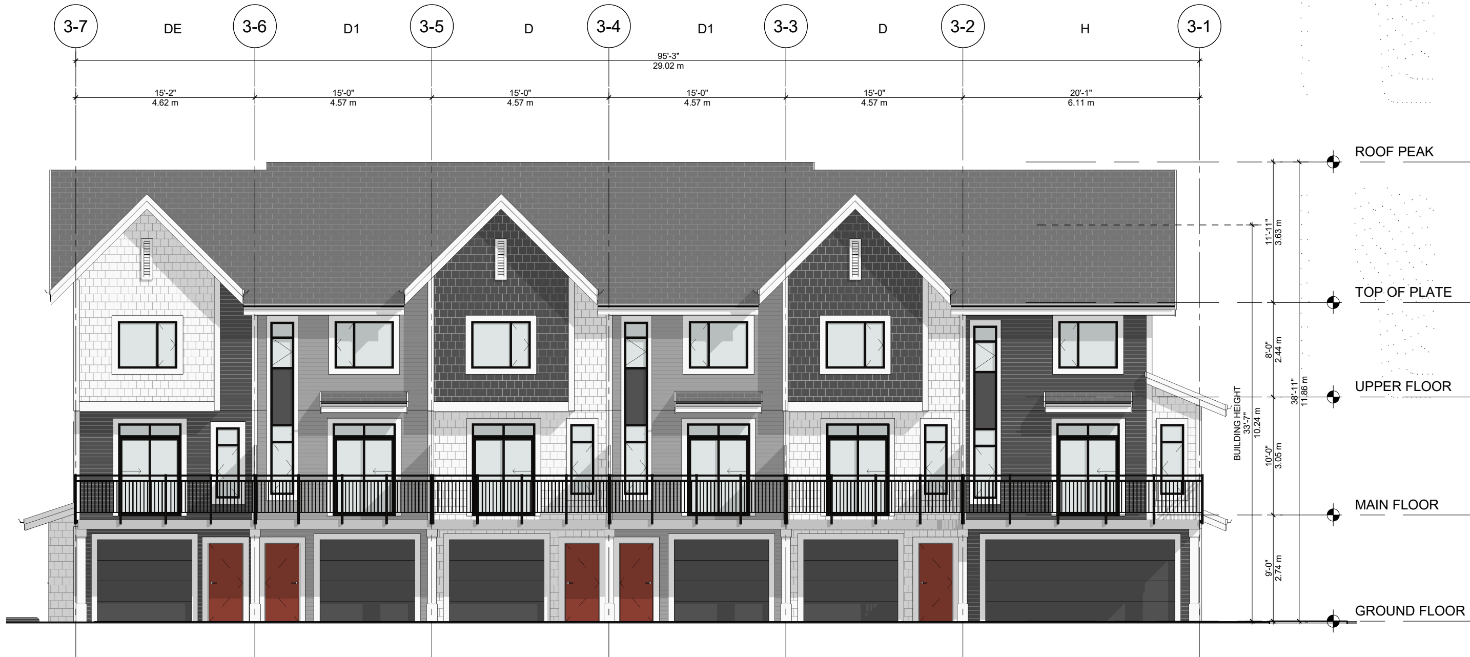
2 NORTH ELEVATION - BUILDING 3 & 16 1 : 100 BUILDING 3 NORTH ELEVATION
