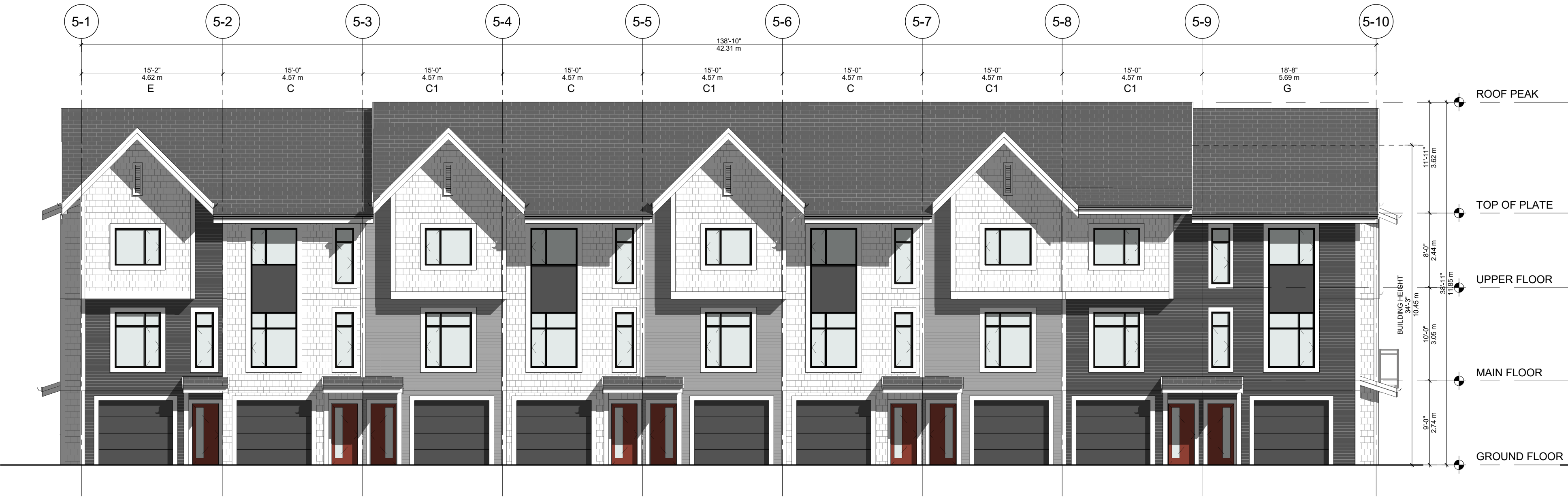
1 SOUTH ELEVATION - BUILDING 5, 6, 9, 10, 13 & 14 1 : 100
